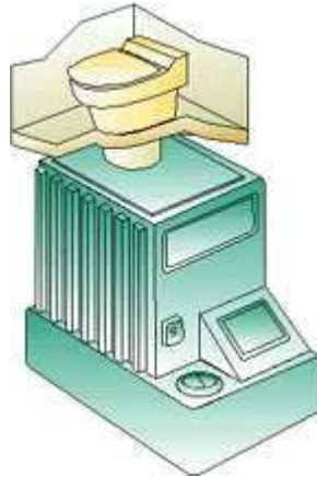
Figure 17 : Clivus Multrum composting toilet (Source: Clivus Multrum)
