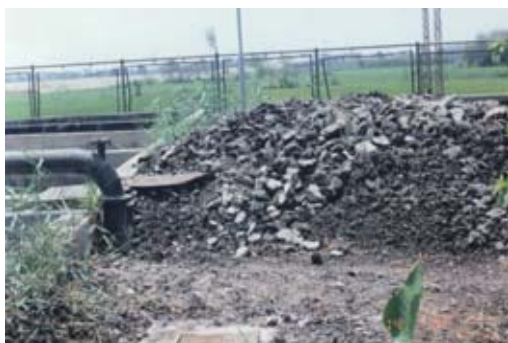
Photo 1: Dried sludge stored besides the drying beds
