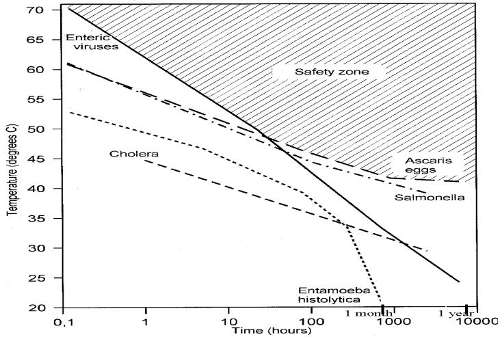
Combination of time and temperature of pathogens elimination. Hatch area represents complete pathogens elimination due to the combined effect of time and temperature (Feachem et al., 1983)
