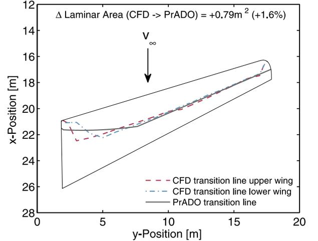
Fig. 3. Comparison of spanwise transition position, PrADO transition model vs. high-fidelity results.
