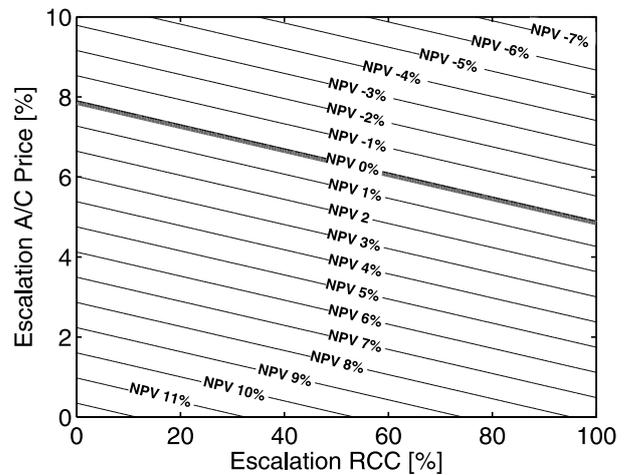
Fig. 13. NPV-isolines for aircraft price variation and RCC cost variation (design range with reduced laminar flow - fuel price scenario 140 US\$/barrel).
