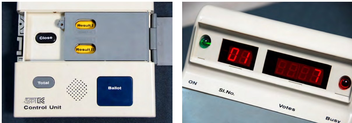
Figure 3: Behind plastic doors there is black close button and result button (left). Display unit on the right (Prasad et al, 2010).
