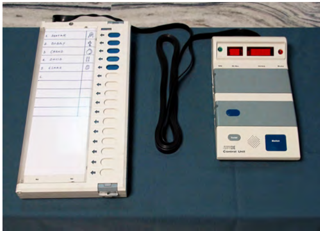
Figure 2: Indian EVM consisting of a ballot unit (left) and a control unit (right) joined by a five-meter cable. (Prasad et al, 2010).
